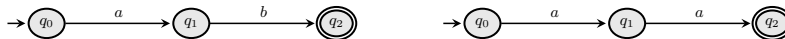
Fig. 2. Deterministic finite automata A_1 and A_2 accepting the bideterministic and finite languages L_1 = \{ab\} and L_2 = \{aa\} , respectively. In both drawings the non-accepting sink state is not shown. The longest simple path in both automata is of length 3 (including the non-accepting sink state) and the pumping constants of the languages are \mathbf{mpe}(L_1) = 3 and \mathbf{mpe}(L_2) = 4 .
